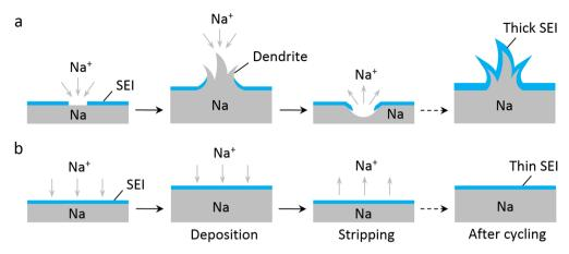
Figure 1. Schematics showing the difference between (a) dendritic and (b) nondendritic Na deposition.
