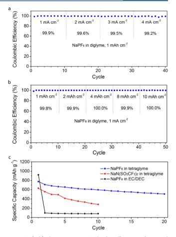
**Figure 6.** (a, b) Plating—stripping Coulombic efficiencies of Na metal anodes cycled using 1 M NaPF $_6$  in diglyme at (a) 1 mAh cm $^{-2}$  with increasing current densities and (b) 1 mA cm $^{-2}$  with increasing areal capacities. (c) Specific capacities (calculated based on the mass of S) of room-temperature Na–S batteries cycled using various electrolytes at 0.1 C (1 C = 1673 mA g $^{-1}$ ) from 1.2 to 2.8 V vs Na $^+$ /Na.
