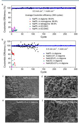
**Figure 3.** (a, b) Plating—stripping Coulombic efficiencies of Na metal anodes cycled using (a) 1 M NaPF<sub>6</sub> in various electrolyte solvents and (b) 1 M of various electrolyte salts in diglyme. (c–f) Low- and high-magnification SEM images of the Na metal surface after 1 cycle at 0.5 mA cm<sup>-2</sup> and 1 mAh cm<sup>-2</sup> using (c, d) 1 M NaPF<sub>6</sub> in 1:1 v/v EC/DEC and (e, f) 1 M NaN( $SO_2CF_3$ )<sub>2</sub> in diglyme.
