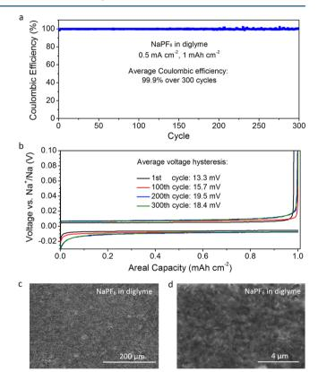
**Figure 2.** (a) Plating—stripping Coulombic efficiencies and (b) voltage profiles and average voltage hysteresis, as well as (c) low- and (d) high-magnification SEM images of Na metal anodes after 1 cycle, cycled at  $0.5~{\rm mA~cm^{-2}}$  and  $1~{\rm mAh~cm^{-2}}$  using  $1~{\rm M~NaPF_6}$  in diglyme.
