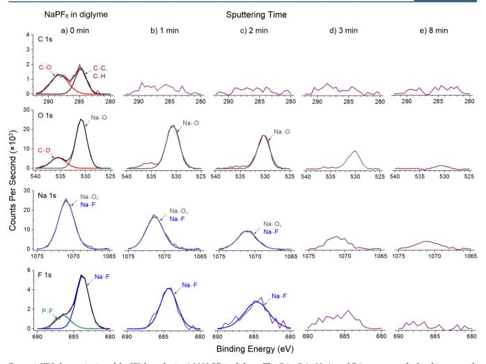
Figure 4. XPS characterization of the SEI formed using 1 M NaPF $_6$  in diglyme. The C 1s, O 1s, Na 1s, and F 1s spectra are displayed in rows, with corresponding depth profiling results in columns after (a) 0 min, (b) 1 min, (c) 2 min, (d) 3 min, and (e) 8 min of sputtering.
