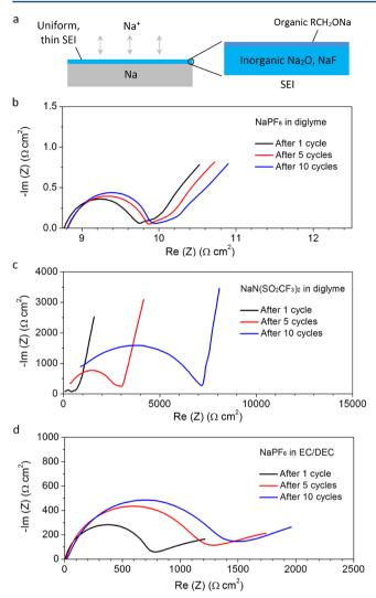
**Figure 5.** (a) Schematic showing the SEI formed on the Na metal surface using NaPF<sub>6</sub> in glymes. (b-d) Impedance spectra of Na metal anodes cycled using (b) 1 M NaPF<sub>6</sub> in diglyme, (c) 1 M NaN(SO<sub>2</sub>CF<sub>3</sub>)<sub>2</sub> in diglyme, and (d) 1 M NaPF<sub>6</sub> in 1:1 v/v EC/DEC.
